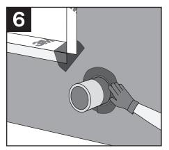
Detail penetrations by wrapping  $3M^{\sim}$  Ultra Conformable Flashing Tape 3015UC around the penetration, ensuring the lap ends at the bottom with a minimum of a 2" overlap.
