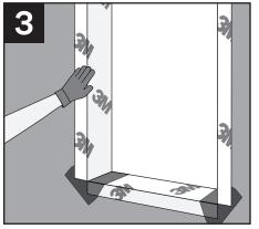
To detail the vertical sides of window, cut 3M<sup>™</sup> Air and Vapor Barrier 3015 the same length as the height of the frame. Extend onto the wall and overlap the sill flashing a minimum of 2" to prevent negative laps.
