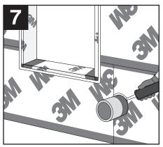
Any negative laps and penetrations need to be caulked after the wall air barrier is applied.
