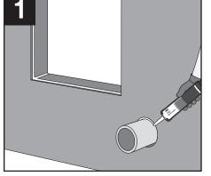
Prep window opening and penetrations. Caulk gaps and ensure all mortar joints are struck flush. Gaps wider than 1/2" must be filled with backer rod and caulk prior to applying  $3M^{\sim}$  Ultra Conformable Flashing Tape 3015UC.
