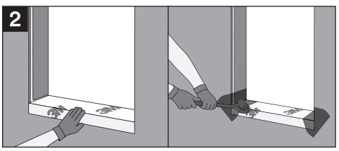
If  $3M^{\mathbb{M}}$  Air and Vapor Barrier 3015 will be used as the sill flashing tape, first cut it the width of the window and apply over the sill extending at least 2" onto the wall. Then apply  $3M^{\mathbb{M}}$  Ultra Conformable Flashing Tape 3015UC in the corners, extending over the sill tape and up the vertical side of the frame ensuring a minimum 2" overlap in all directions. Apply pressure with a J-roller.
