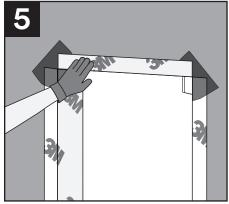
To complete the window detailing, cut a piece of  $3M^{\circ\circ}$  Air and Vapor Barrier 3015 the same width as the window. Overlap a minimum of 2" onto the wall and over the  $3M^{\circ\circ}$  Ultra Conformable Flashing Tape 3015UC in the upper corners.
