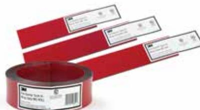
3M™ Fire Barrier Tuck-In Wrap Strips are designed for use with PVC, PVCc, PE and PP plastic pipes penetrating through concrete floors, block and concrete walls, and gypsum stud walls. Wrap Strip easily slides into annular space and is topped with 3M™ Fire Barrier IC 15 WB+ and 3M™ Fire Barrier Watertight Silicone 3000 WT Sealant.
