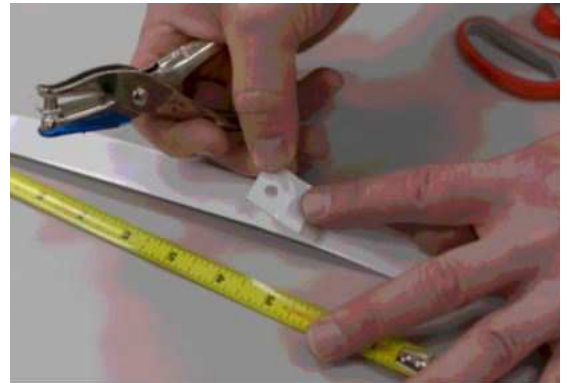
Figure 2. Preparing the test strips
