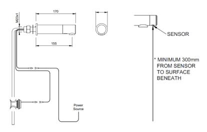
PLEASE NOTE: Dolphin recommends having access available to the fixing nut on the back of the tap for installation & ongoing maintenance. Maintenance of the tap solenoid and diaphragm should also be addressed every 6 months. Further details are provided in the maintenance booklet supplied with each sensor tap.
