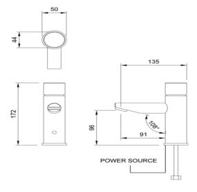
PLEASE NOTE: Dolphin recommends having access available to the fixing nut on the back of the tap for installation & ongoing maintenance. Maintenance of the tap solenoid and diaphragm should also be addressed every 6 months. Further details are provided in the maintenance booklet supplied with each sensor tap.
