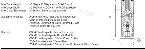
On-Eazi CDS42 Series Bottom Rail Module to suit Pivot Bearing or BTS Floor Spring Applications with Lock
