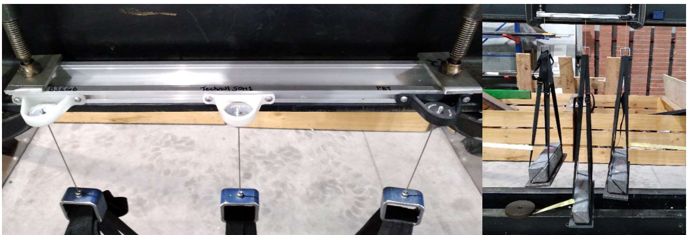
Figure 2 - Sidemount clips under static load
