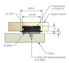
Through section showing surface mounted adhesive installation
