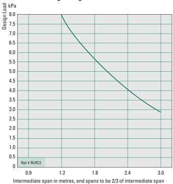
Testing confirms that .70mm Aluminium has similar results to .40mm Steel and that .90mm Aluminium has similar results to .55mm Steel and is adjusted for practical application.
