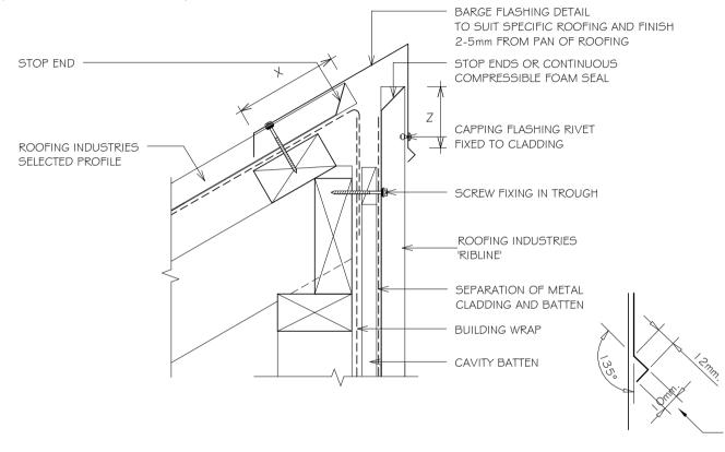
BIRD'S BEAK at bottom edge of vertical flashing Detail Number: RI-RRW002B-1
