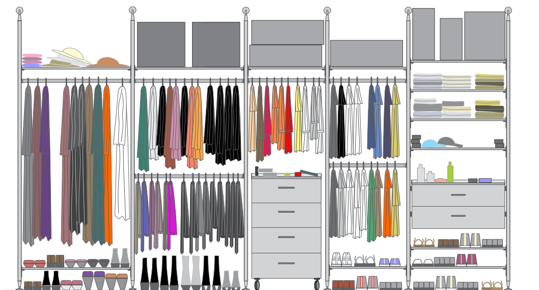
Typical Elevation - Clothing, Storage, Side1 (Her side) Shelving 500mm deep, Drawers 500mm deep
