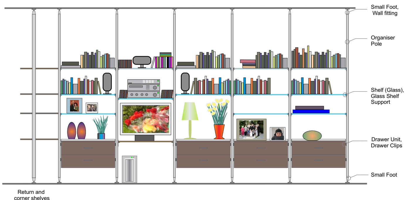
Typical Elevation -Living, Entertainment Area Shelving 300mm deep, Drawers 500mm deep
